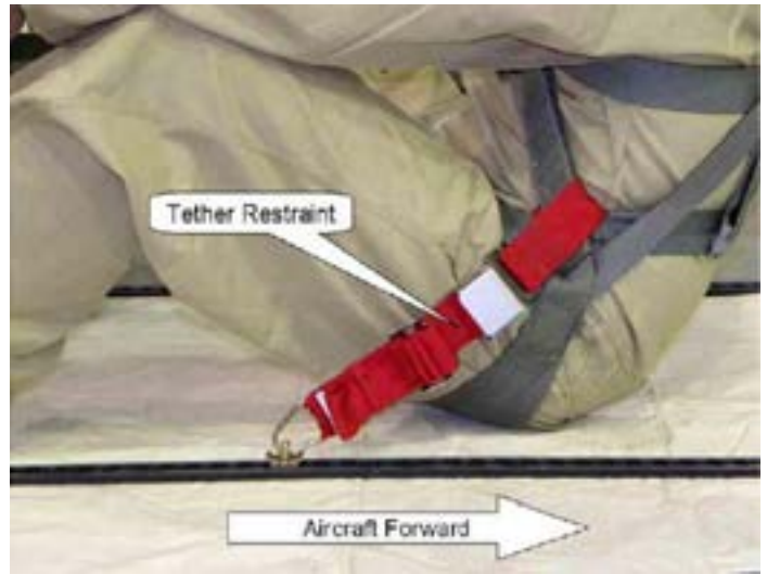
Figure 7. Tether Restraint Attachment To Floor For Rear-Facing Floor Seats
