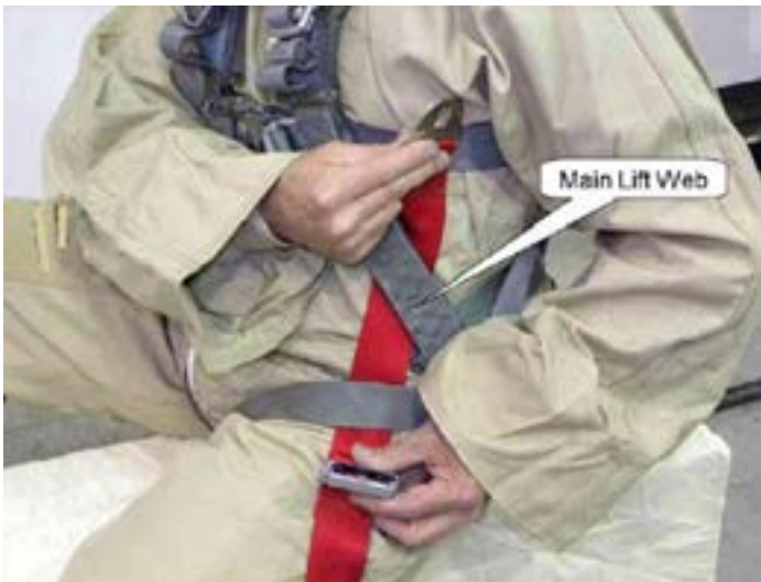
Figure 5. Pass Tether Loop Under Main Lift Web
