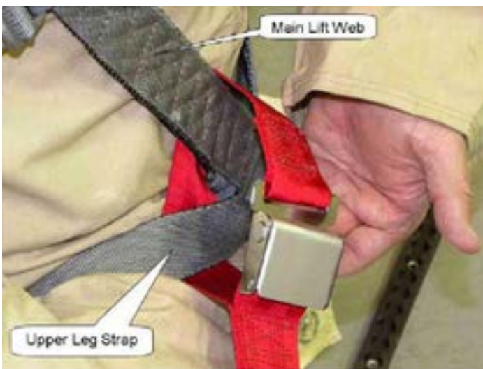
Figure 6. Latch Tether Loop Around Parachute Harness
