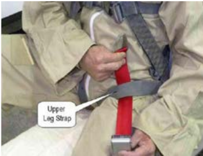
Figure 4. Pass Tether Loop Under Upper Leg Strap
